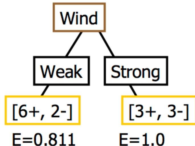
$$\begin{aligned} \text{Gain}(S, \text{Wind}) &= 0.940 - (8/14) * 0.811 \\ &\quad - (6/14) * 1.0 \\ &= 0.048 \end{aligned}$$
