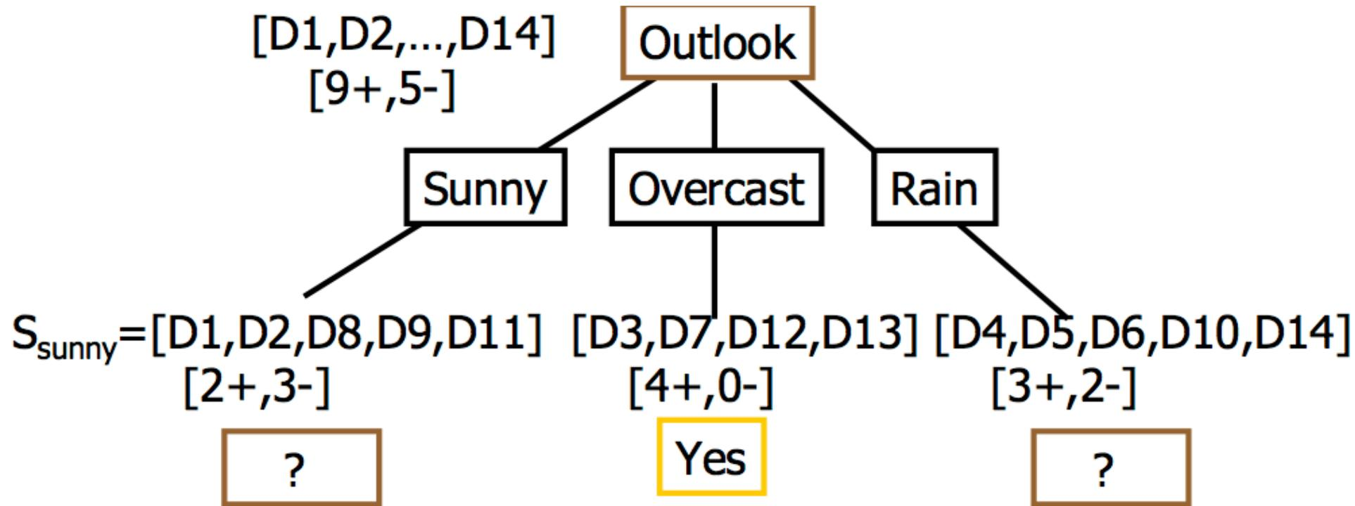
$$\text{Gain}(S_{\text{sunny}}, \text{Humidity}) = 0.970 - (3/5)0.0 - 2/5(0.0) = 0.970$$
