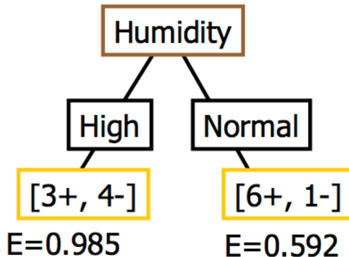
$$\begin{aligned} \text{Gain}(S, \text{Humidity}) &= 0.940 - (7/14) * 0.985 \\ &\quad - (7/14) * 0.592 \\ &= 0.151 \end{aligned}$$
